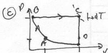
$\phi = \delta Q_{AB} + \delta Q_{BC} + \delta Q_{CD} + \delta Q_{DA} + \delta W$
