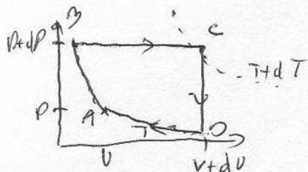
$$\Delta U = (c_p dT + h dP)_{AB} + (c_p dT + h dP)_{BC} + (c_v dT + l dV)_{CD} - (c_v dT + l dV)_{DA} + W = 0$$
