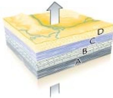
Continual erosion strips D away completely and exposes C to erosion
